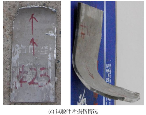
(c) 试验叶片损伤情况 图 13 试验叶片损伤情况与数值仿真相比较 Fig.13 Damage of testing blade compared with the numerical simulation
