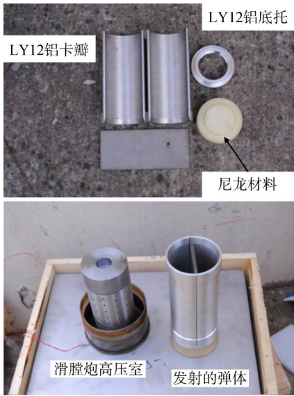
图 3 滑膛炮高压室和弹体 Fig.3 Bombard high-pressure chamber and projectile
